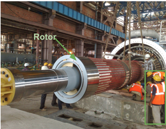
FIG. 19. Image of generic generator. Rotor is very massive and consequently has a large moment of inertia 25 .
